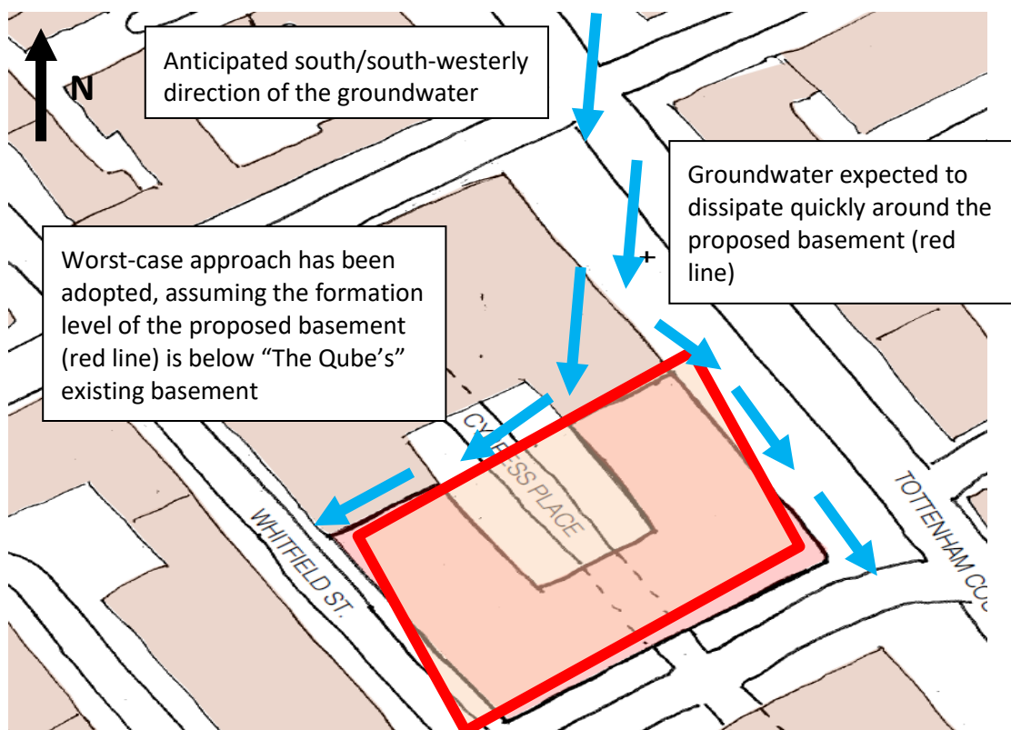
Plate 1. Anticipated groundwater flow post-construction of the proposed redevelopment (blue: potential groundwater path; red: indicative site boundary for The Network Building)
