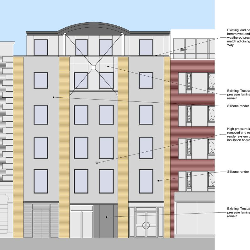
Existing lead parapet cappings to beremoved and replaced with 'Once-- weathered precast concrete copings' to match adjoining building at 141-143 York
