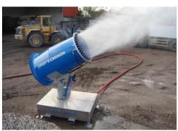
Purpose built dust suppression cannons will be used throughout the demolition phase to damp down areas and minimise airborne dust particles.
