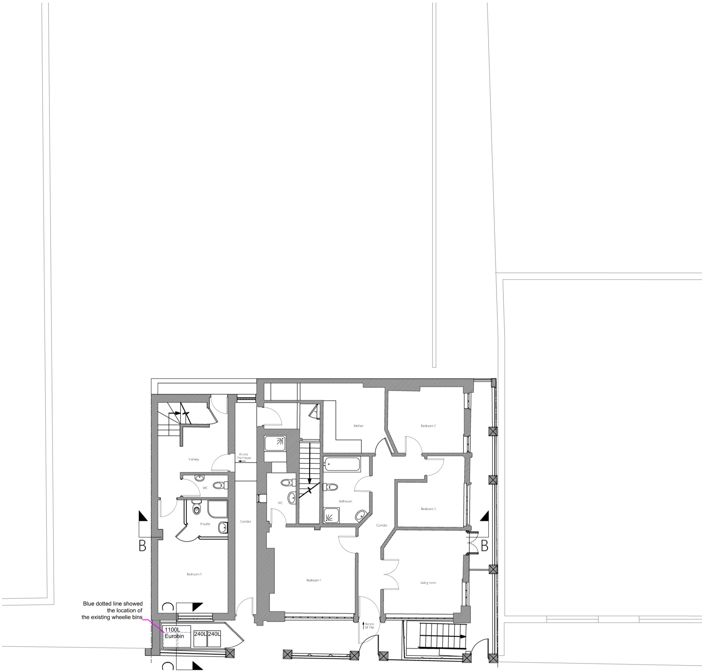
PROPOSED GROUND FLOOR PROPOSED BIN STORAGE AND CYCLE STORAGE LOCATED IN BASEMENT, NEW STAIRS DOWN TO BASEMENT LEVEL EXTERNALLY TO INCORPORATE A CYCLE WHEEL CHANNEL TO ALLOW EASE OF ACCESS
