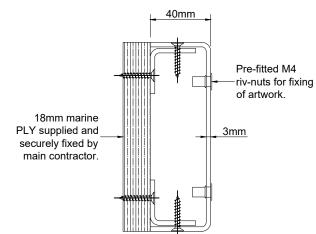
Back panelling to be minimum 3mm aluminium. To be either stove enamalled or powder coated, RAL 9005 (black) satin finish.
