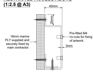
Back panelling to be minimum 3mm aluminium. To be either stove enamalled or powder coated, RAL 9005 (black) satin finish.
