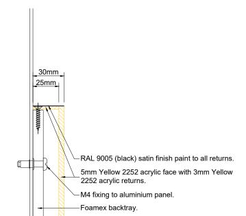
Text "SLOTS" to be built up 5mm Yellow 2252 face with 3mm Yellow 2252 returns. Returns to be sprayed RAL 9005 (black) satin finish. Text to have full router cut foamex backtray and installed flush with background.
