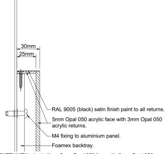
Text "MERKUR" to be built up 5mm Opal 050 face with 3mm Opal 050 returns. Returns to be sprayed RAL 9005 (black) satin finish. Text to have full router cut foamex backtray and installed flush with background.
