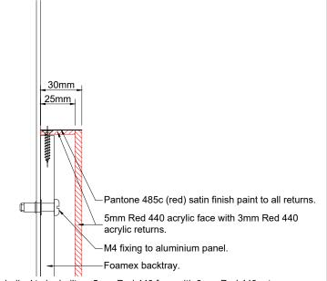
'Underline' to be built up 5mm Red 440 face with 3mm Red 440 returns. Returns to be sprayed Pantone 485c (red) satin finish. Underline to have full router cut foamex backtray and installed flush with background.
