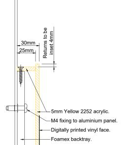
"Sun" logo to be built up 5mm Yellow 2252 acrylic. Face digitally printed onto white vinyl and applied centrally. Logo to have full router cut foamex backtray and installed flush with background.
