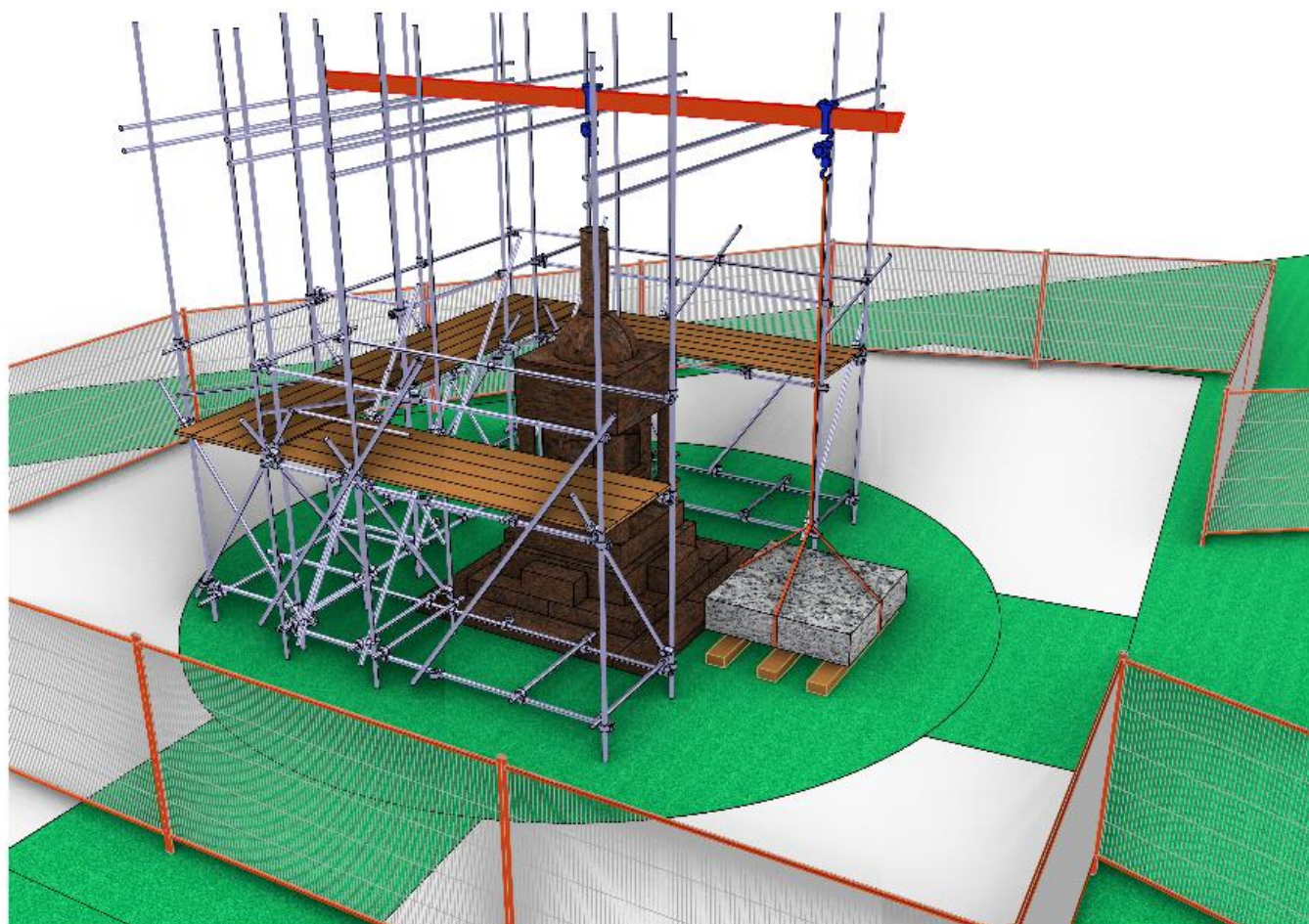
Concept design for scaffolding and lifting process.
