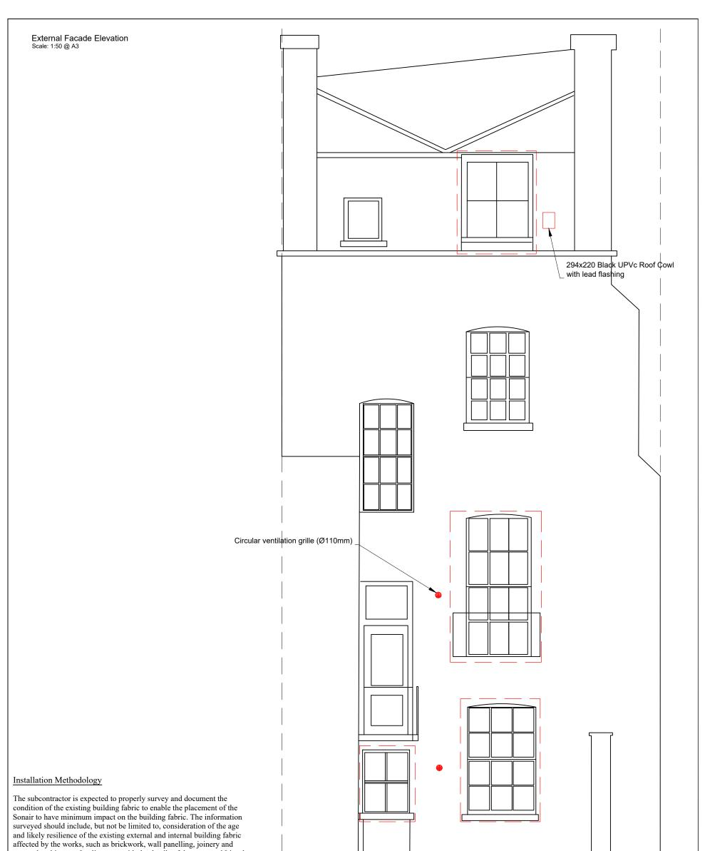
external architraves. In alignment with the details of the approved Listed Building Consent, the subcontractor is required to set-out the position of the ventilation system on site. The positions are to be agreed with CSjv Built Heritage Consultant prior to the commencement of the works. Further details of the proposed penetration process are to be agreed with CSjv Built Heritage Consultant prior to the commencement of the works.
