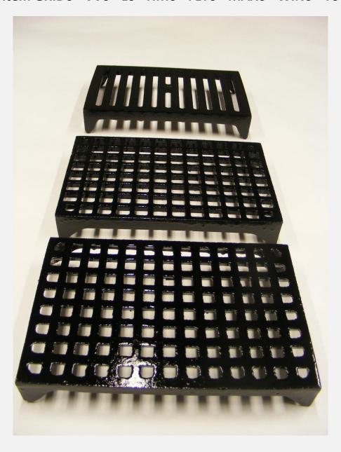
Cast iron air bricks are made from grey iron, cast in sand moulds bonded with resin to a fine cast finish. They are available in numerous sizes and are grouped according to the number of bricks they replace ie, single, double and triple and 12x6 inch. Here we look at the eight different types of double air bricks we have in the range and the photo above is an example from top to bottom of ... Victorian vertical slotted air brick (VV6), maximum air (MAX6) and grid pattern (GRID6)
