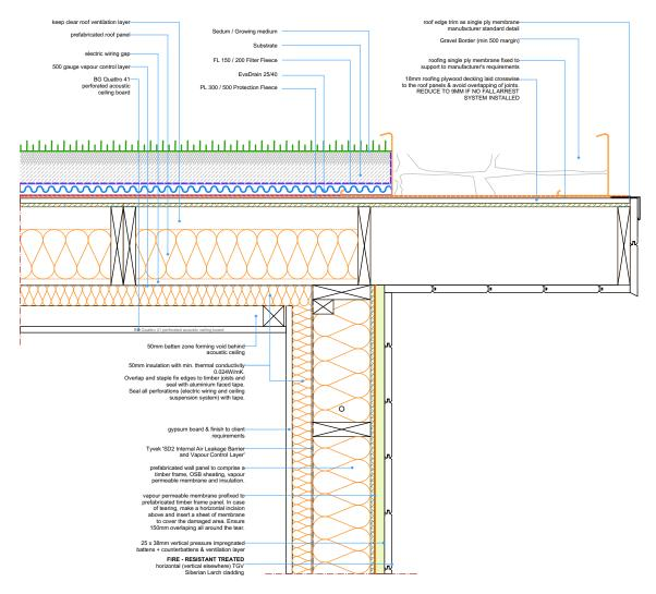
monopitch roof to side wall junction (horizontal cladding)
