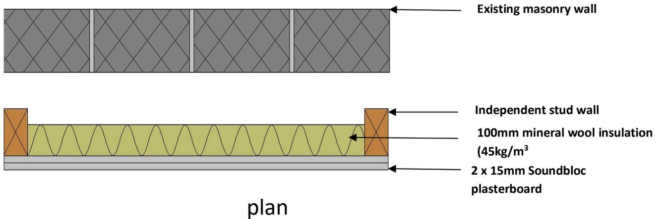
Minimum gap between the existing wall and stud should be at least 10mm.
