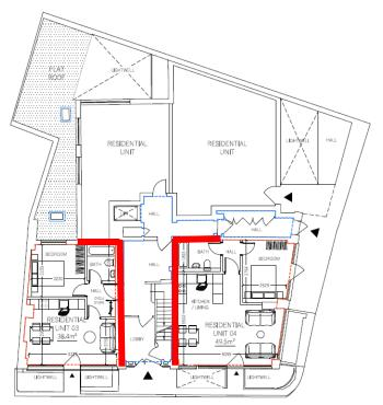
Independent wall lining, 2 x 15mm Soundbloc Plasterboard
