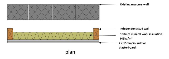
Minimum gap between the existing wall and stud should be at least 10mm.
