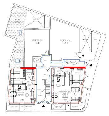
100mm independent stud filled tightly with 100mm mineral wool insulation (45kg/m<sup>3</sup>), 2 x 15mm Soundbloc plasterboard either side.
