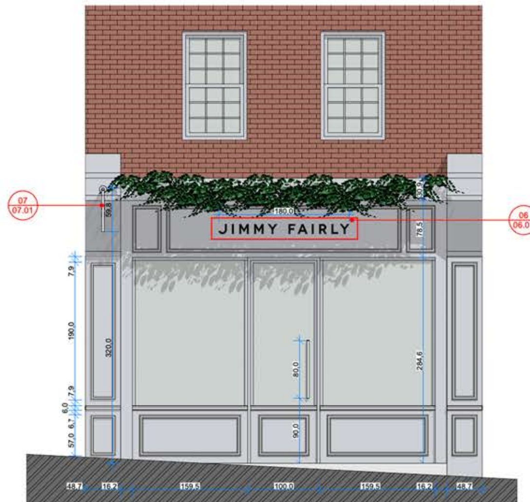
06.02 MAIN SIGNAGE IN CONTEXT Sc: 1:50 ELEVATION
