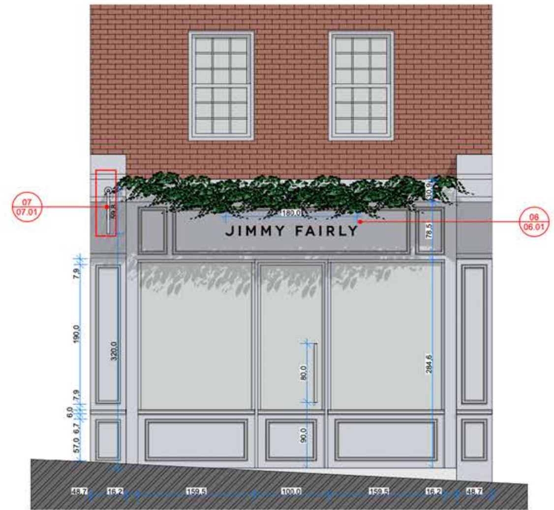
07.02 PROJECTING SIGN IN CONTEXT Sc: 1:50 SECTION & ELEVATION
