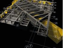
3 White Collar Factory: Models (3D and analytical) showing both the LUL and Network Rail subterranean tunnels running below and adjacent to the building
