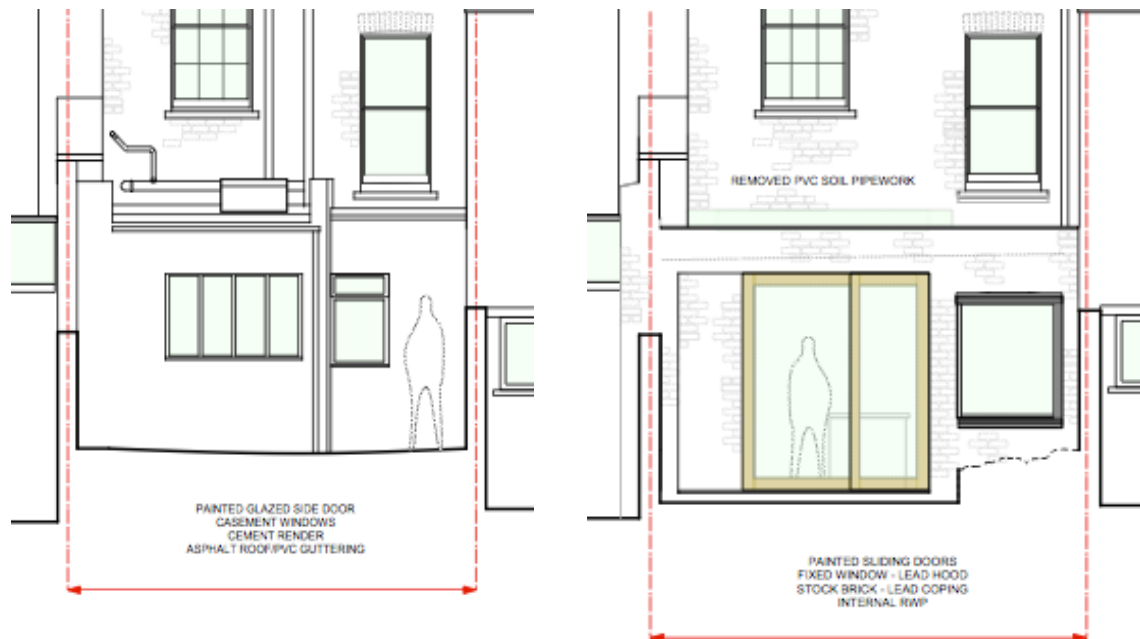
Figs. 8 & 9 Existing and Proposed rear elevations, replacing cement render with London stock brick and rationalizing external pipework.
