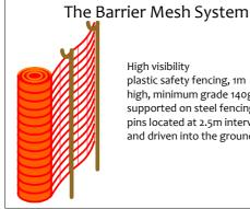
High visibility plastic safety fencing, 1m high, minimum grade 140g/m2, supported on steel fencing pins located at 2.5m intervals and driven into the ground.
