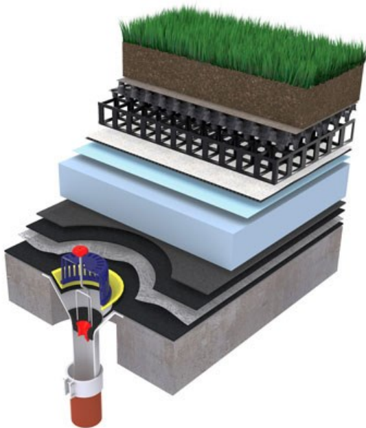
Figure 5 Alumasc typical green roof build-up
