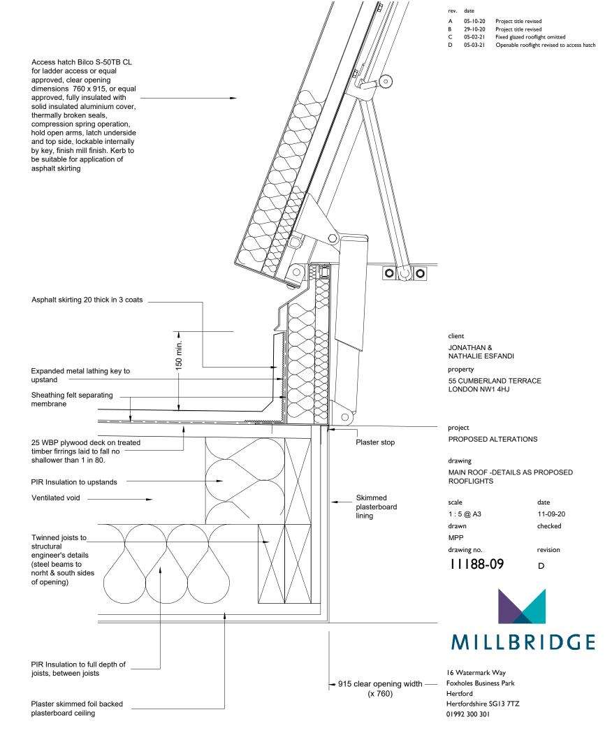
Detail 2- main roof, part section through openable rooflight
