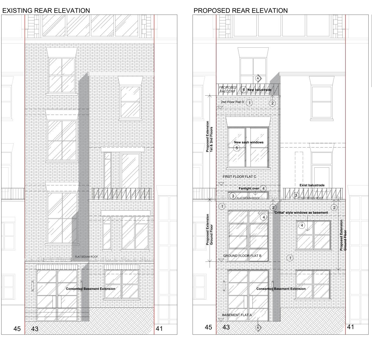
New Brickwork - London stock reclaimed second hand brickwork to match the existing.
