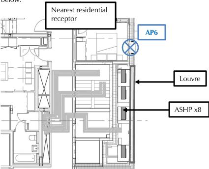
5.4.2 It will be necessary for the louvre to be acoustically rated, so to achieve the following insertion losses:
