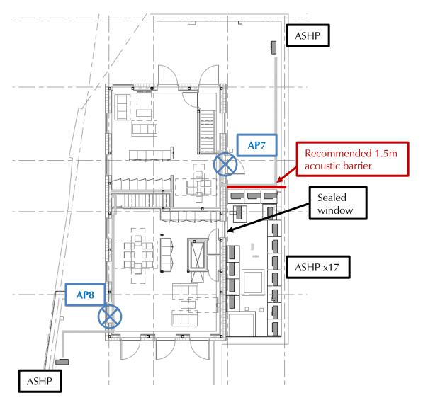
5.5.2 The apartment window overlooking the plant area is proposed to be sealed and tripled glazed, such that internal levels will be controlled through the glazing system. Therefore, noise levels
