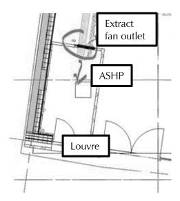
5.3.7 Noise levels have been calculated from the plant room through the louvre to the window of the residential apartment proposed directly above at 1<sup>st</sup> floor (AP4).
