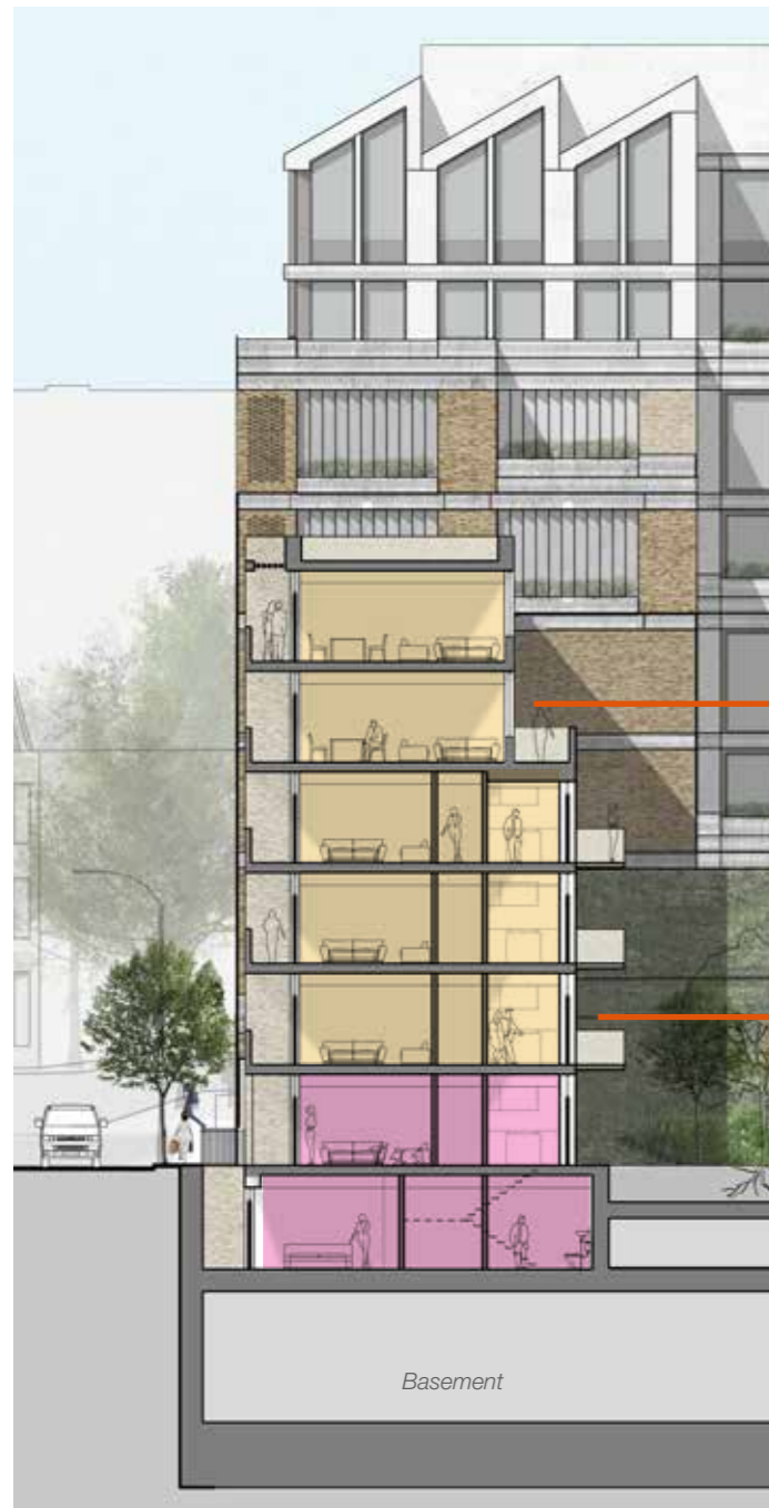
A gallery accessed building
