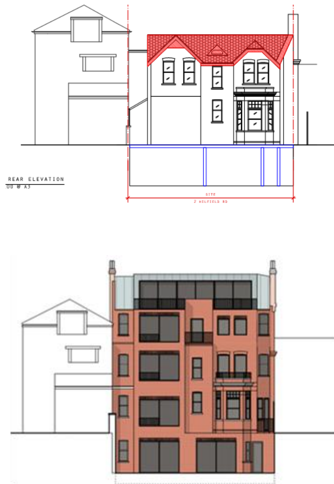
Figure 9: Existing and proposed rear elevations
