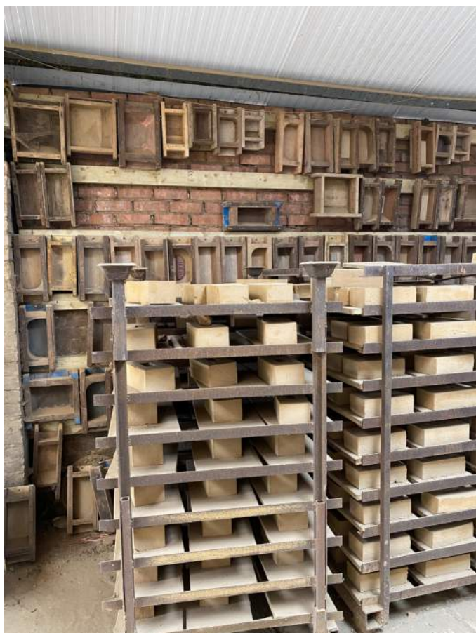
Photographs of hand made bricks drying at H G Matthews, and close up of clay strocks (cob blocks used for new internal walls)
