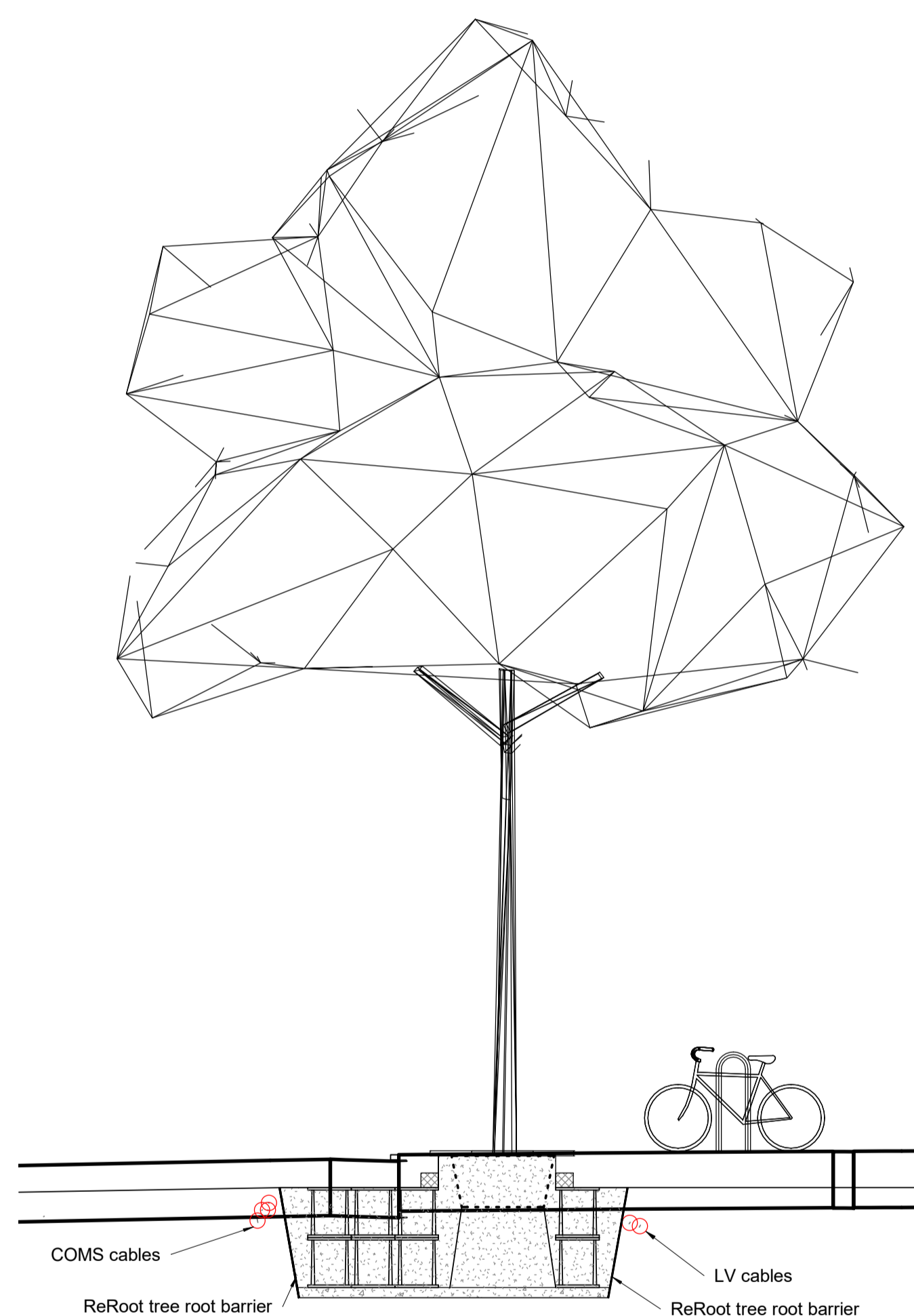
First tree (North) Landscape tree pit section Indicative tree pit with soil cells and root barrier between existing services. SCALE 1:50@A1
