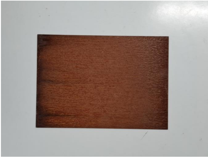
Photographs 1 and 2: Weathered Corten Steel (sample weathered for 12 months)
