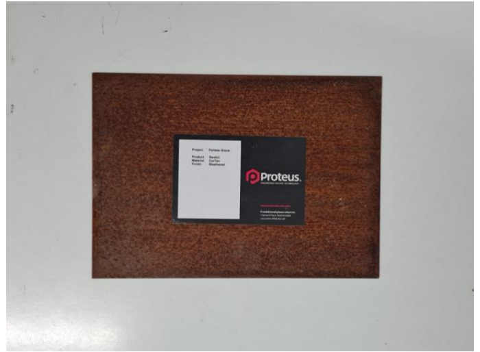
Photographs 1 and 2: Weathered Corten Steel (sample weathered for 12 months)
