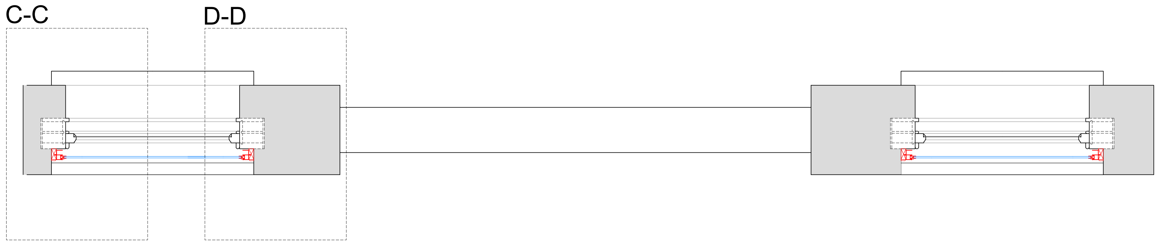
Plan Section B-B with Secondary Glazing Installed Scale: 1:10
