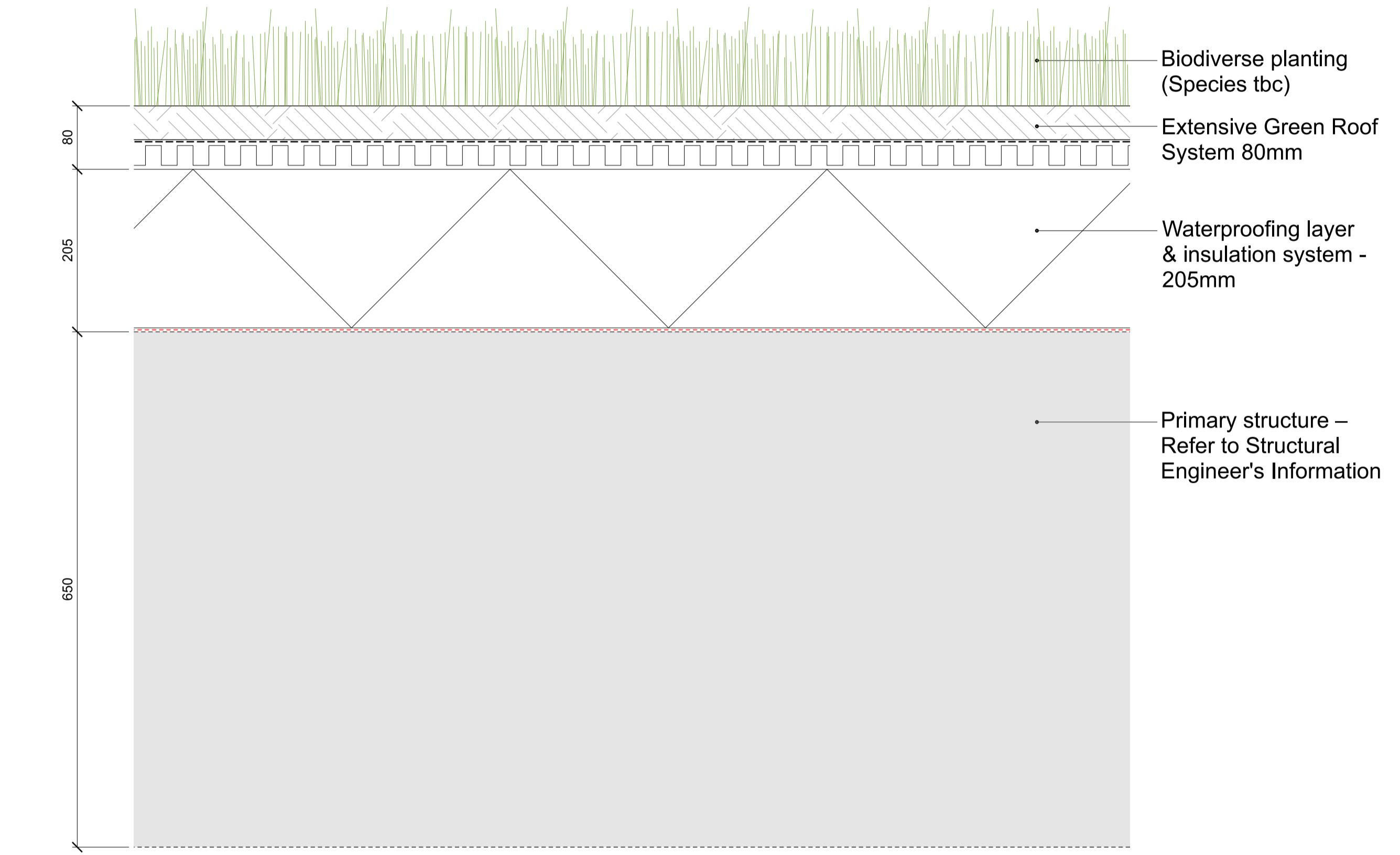
02 DETAIL: EXTENSIVE GREEN ROOF (80mm SUBSTRATE)
