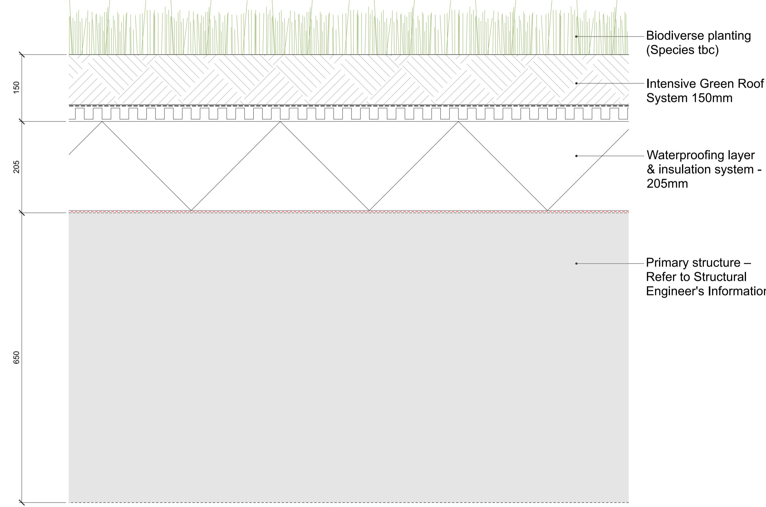
01 DETAIL: INTENSIVE GREEN ROOF (150mm SUBSTRATE)
