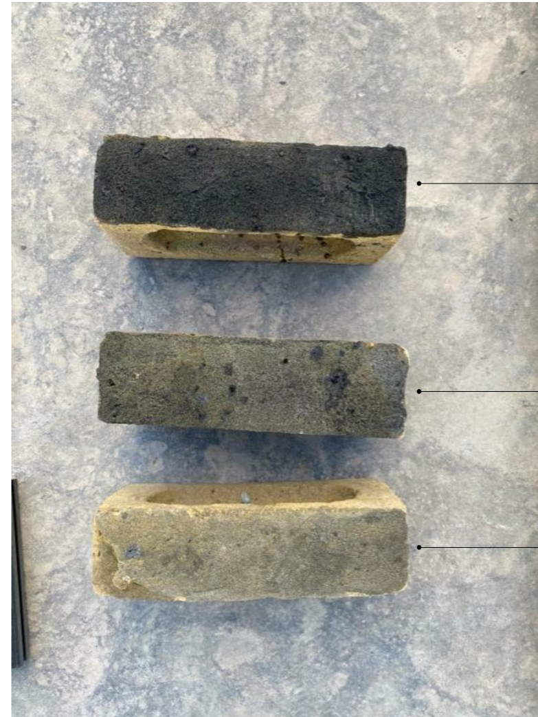
Material samples on site of the varying levels of sootwashing to be confirmed in writing by the local planning authority.
