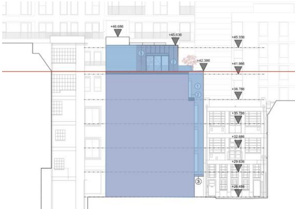
Annotated extract of drawing 303 submitted with the current application - blue shading highlights the main bulk of the building, red line marks the height of the main bulk of the building approved in 2012 (as shaded blue on drawing 233/PD/312 above)
