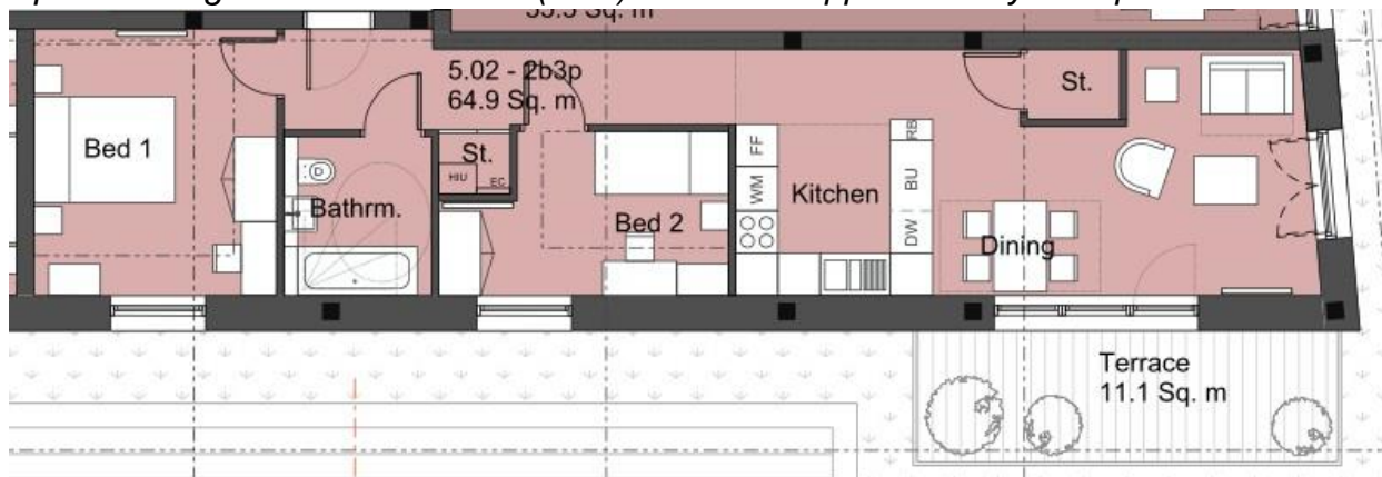
Extract of drawing 105 - 2b3p flat on the fifth floor. This unit has policy-compliant outdoor space. Nonetheless, the LKD measures approximately 29 sqm
