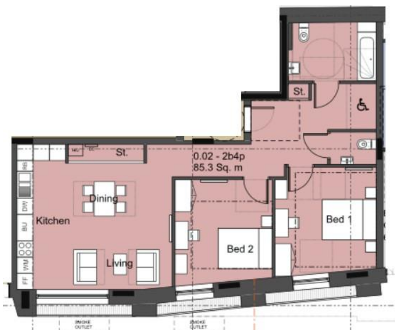
Extract of drawing no. 100 - 2b4p disabled persons' flat on the ground floor. No outdoor space is provided in any form.
