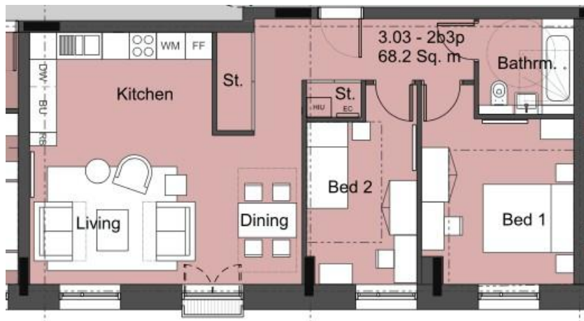
Extract of drawing 103 - 2b3p flat on the third floor. This unit has no countable outdoor space. Living room/kitchen/diner (LKD) measures approximately 30 sqm
