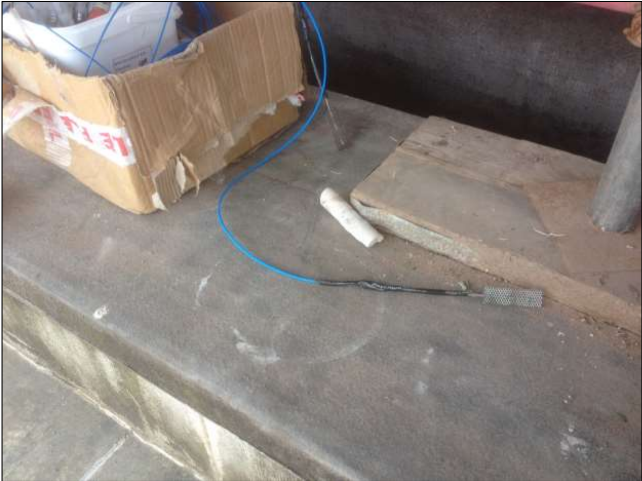
Photograph 4 – A decay probe on site ready for installation.
