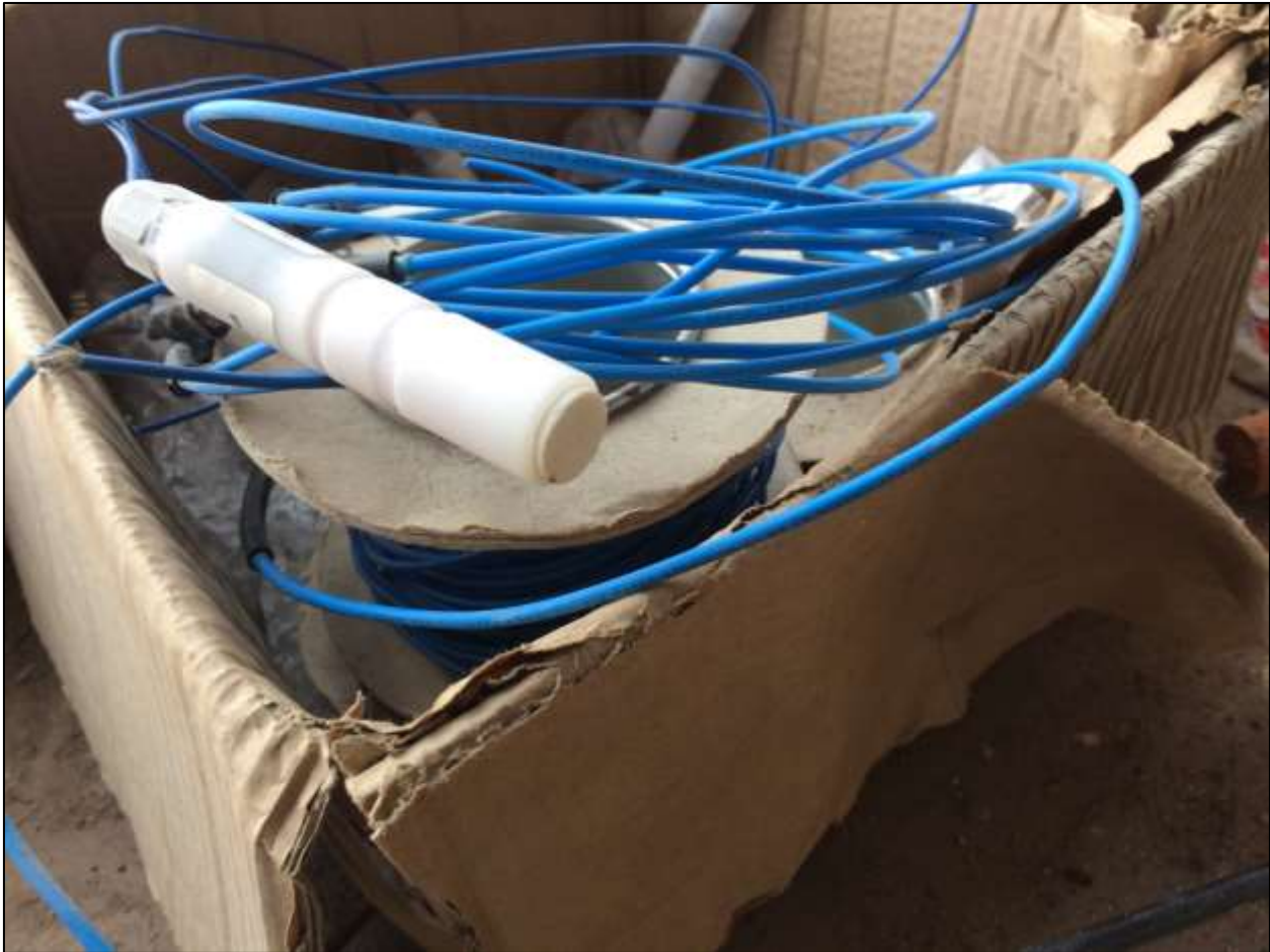
Photograph 3 – A close up view of a single reference electrode [with cap removed] prior to installation.
