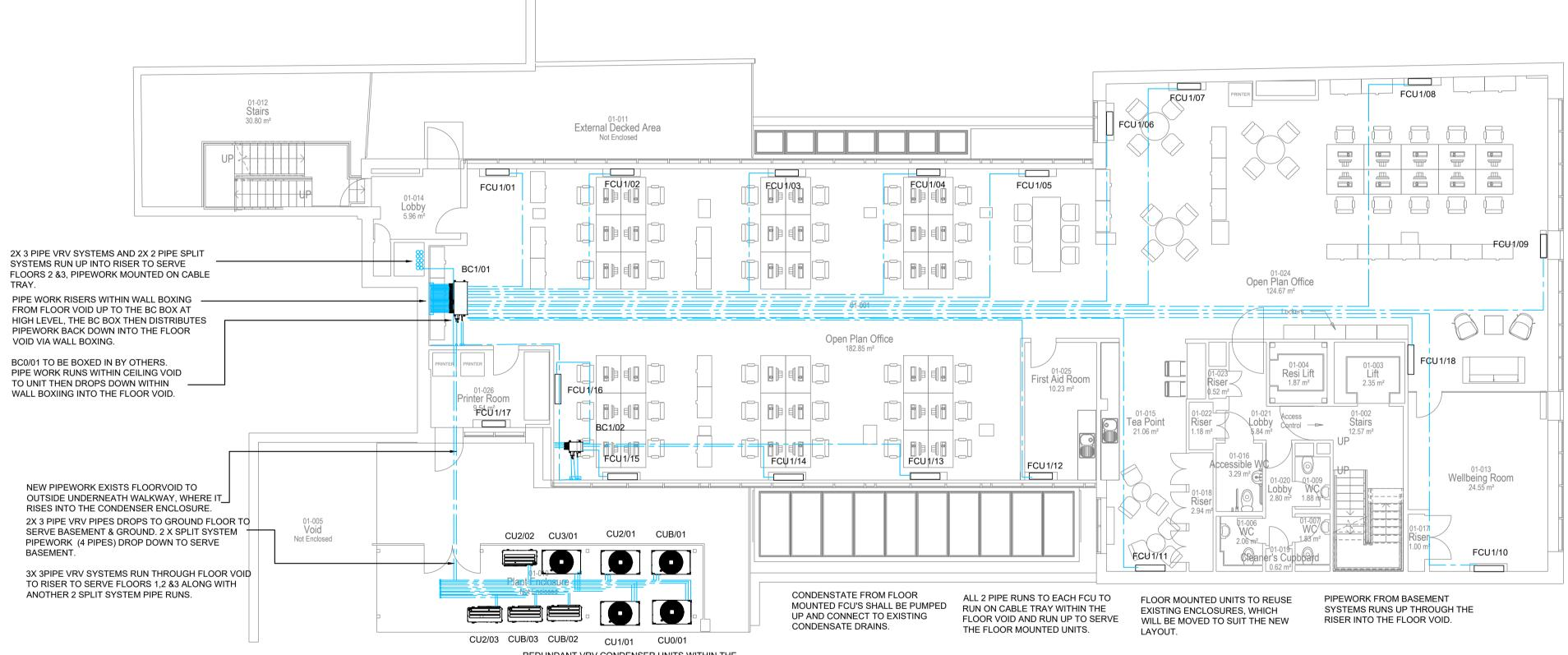
REDUNDANT VRV CONDENSER UNITS WITHIN THE ACOUSTIC ENCLOSURE TO BE REMOVED AND REPLACED WITH NEW.
