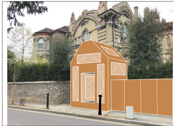
Plywood sheathing to all framed up faces of the historic arch and incl both sides and top of the boundary wall. Access panels to be openable to allow weekly movement monitoring and recording. No access for contractors permitted through archway during the construction works
