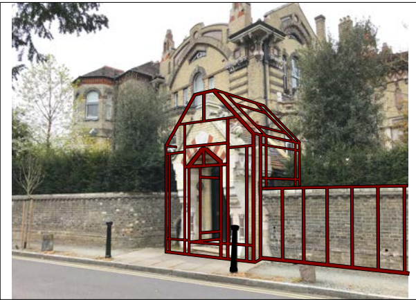
Self supporting timber frame work constructed away from but surrounding the Archway complete, incl the stone steps within and continuing along pavement wall. The profiles timber supporting the underside of the arch to be cushioned. Framed up openings are provided as shown to permit regular movement monitoring
