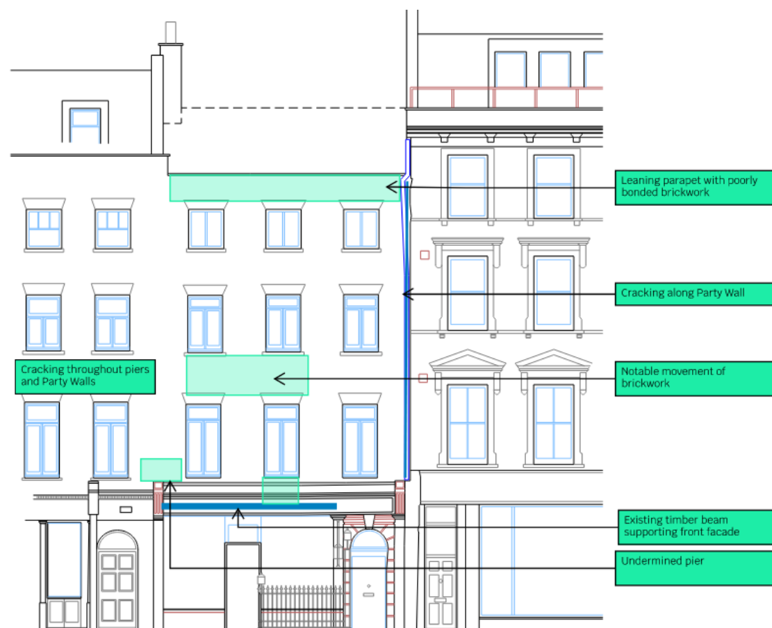
Figure 11 – Summary of front facade defects
