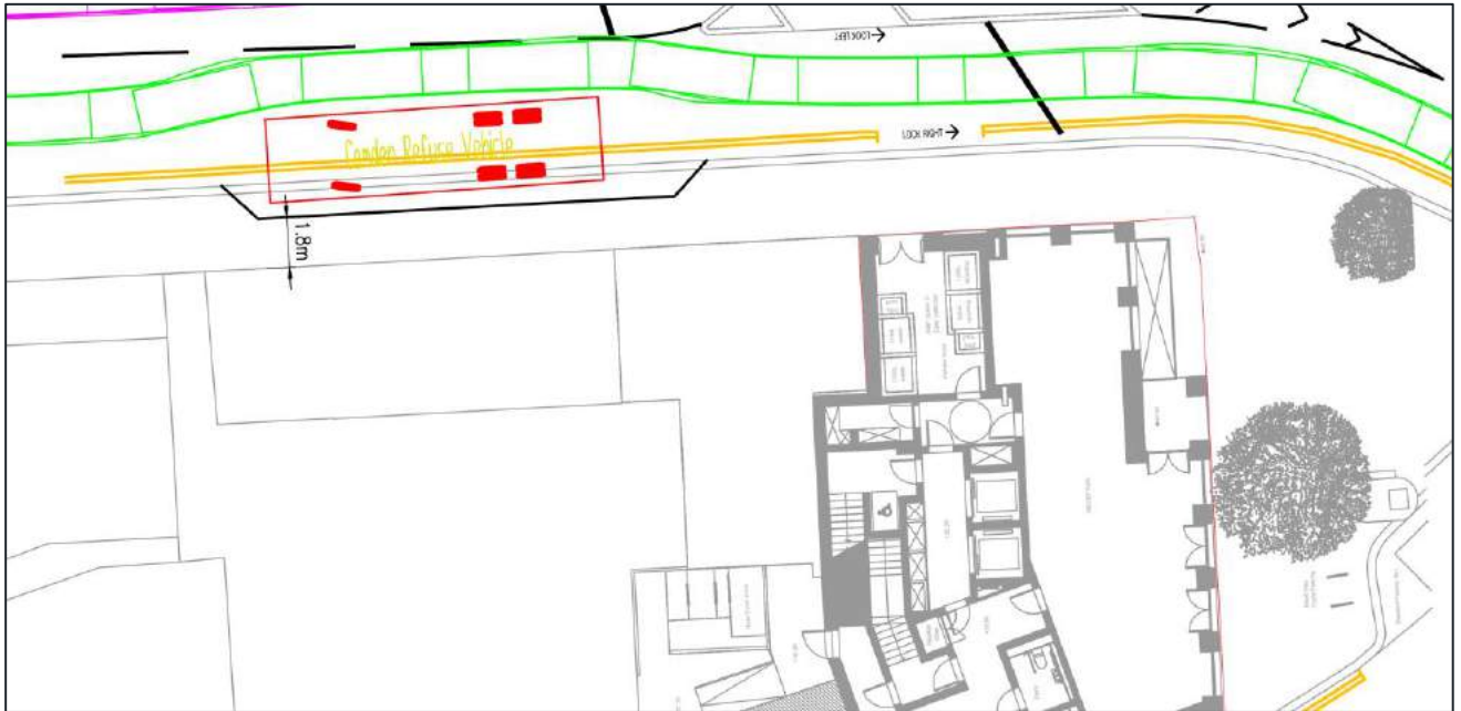
Figure 6-5 Proposed Servicing Arrangements
