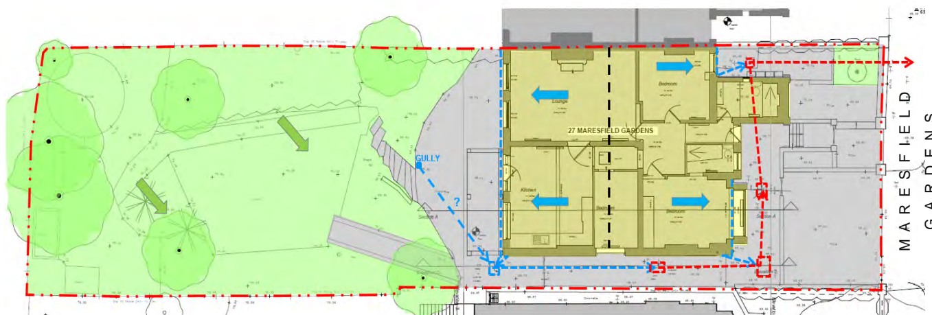
EXISTING SURFACE WATER DRAINAGE LAYOUT
