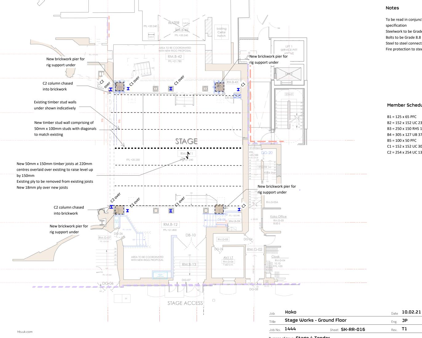
To be read in conjunction with HTS drawings and specification Steelwork to be Grade S355 Bolts to be Grade 8.8 Steel to steel connection design by others Fire protection to steelwork by others
