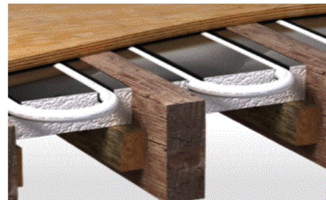
Image 16: Proposed underfloor heating pipes and insulation below Living Room floor. In joist foil boards require fixing of battens only to sides of existing joists and no fixing to top of joists, such as is required by the use of aluminium spreader plates. Thus the top of the existing joists will be unimpeded by the installations and re-fixing of existing floorboards can proceed once the proposed below floor and necessary remedial works are completed.
