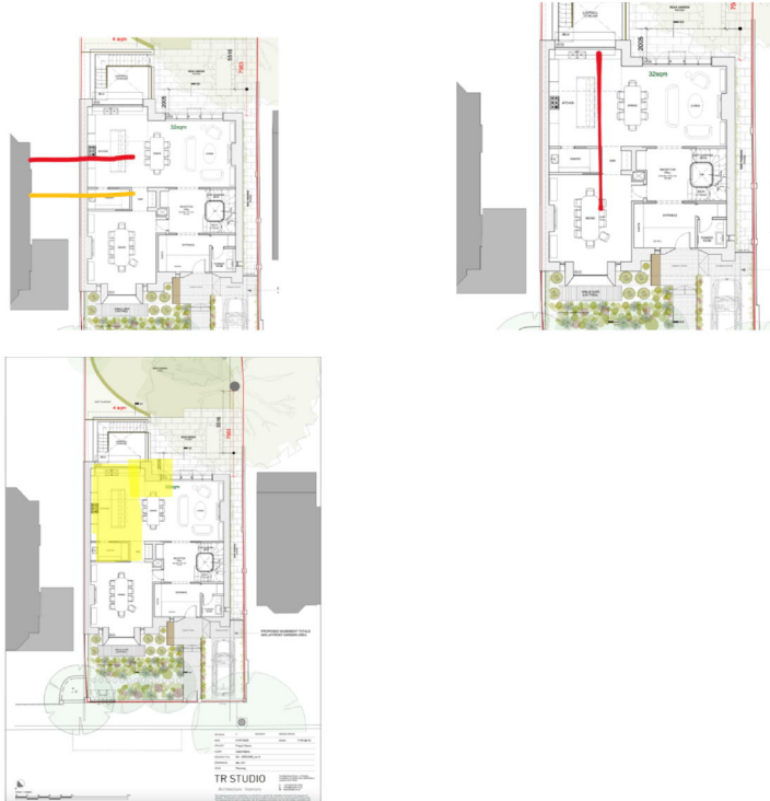
Figure 7 (i) Left. Cutbacks from the rear of the proposed development which would respect the side window (red) or relate to the existing rear wall (yellow) (ii) Right cutback from the side boundary which would mirror the alignment of no 5 Prince Arthur Road (iii) Area of building that would have to be removed to relate to (i) and (ii) and reasonably mirror no 5.
