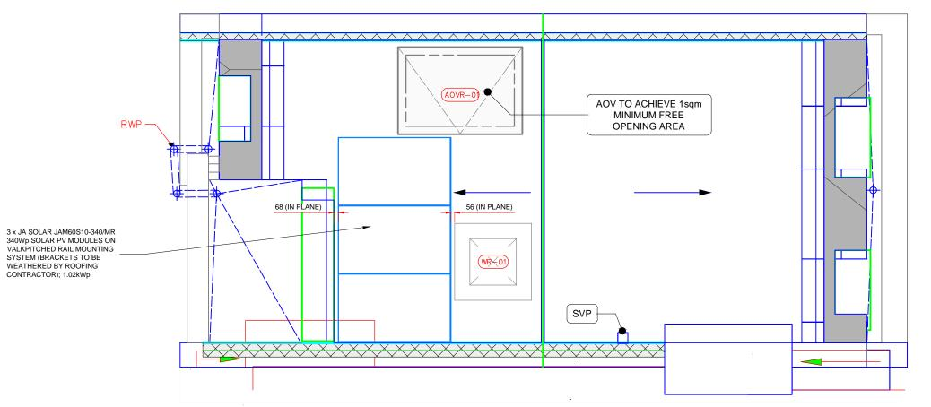
TOTAL SYSTEM: 3 x 340Wp JA SOLAR JAM60S10-340/MR PV MODULES (1689 x 996 x 35mm); 1.02kWp
