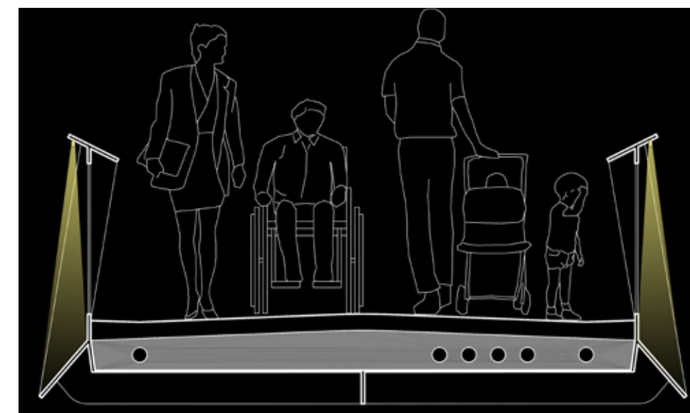
Intended Light Distribution from the Linear LED Under the Handrail
