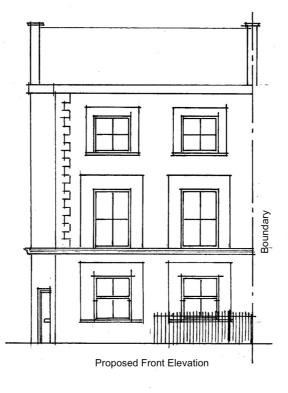
Existing shop front to be relaced with masonry walls with a rendered finish and painted white to match existing.
