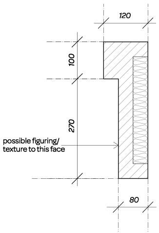
TYPE A forms string course along base of timber clad 1st floor wall, supported by beam or SIP panel behind (requires fixing detail), requires some insulation backing
