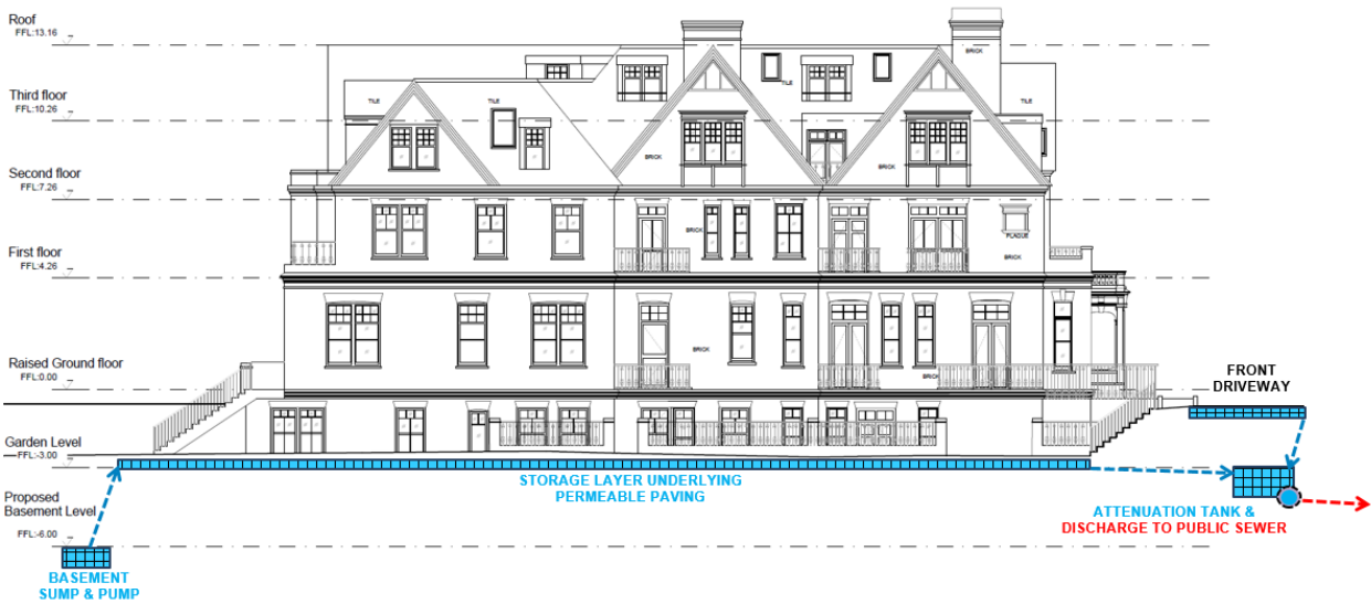
Schematic section showing the approximate arrangement of the proposed attenuation storage SuDS features, showing the levels of the features in relation to each other.
