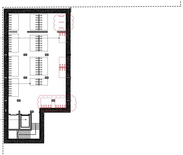
\_\_\_\_\_ 38no. proposed bike storage spaces in double stacked configuration. 3no. bike spaces in Sheffield Cylce Stand configuration, and 3no. bike spaces to be provided at street level as per the Landscape Architects design. Stacked bike storage to match existing 2-tier Josta bike racks
