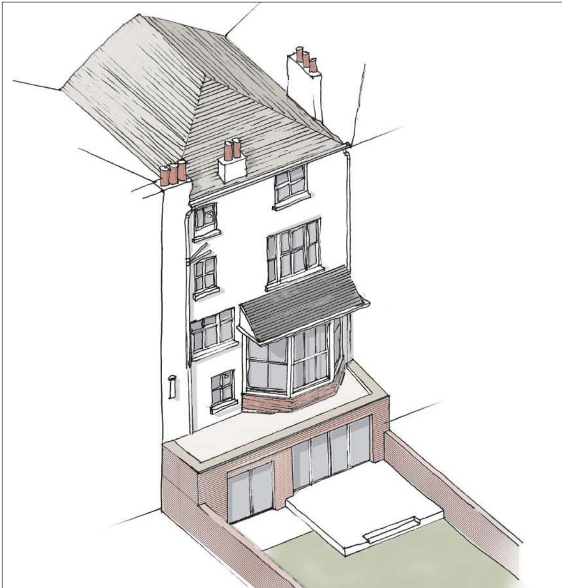
Fig 1: An isometric sketch view of the permitted garden level rear extension.
