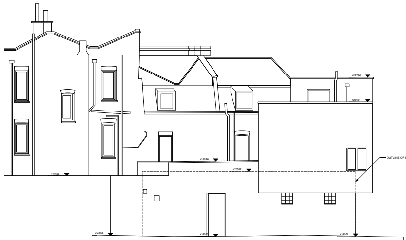
Existing Elevation of neighbouring Building to East @ 1:200 scale
