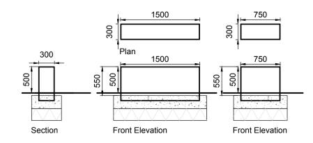
F2 Bespoke Concrete Block MANUFACTURER: CED RANGE: Granite stone PRODUCT REFERENCE:Bespoke cut stone WEBSITE: www.cedstone.co.uk MATERIAL: Granite FIXING: Set on concrete foundation
