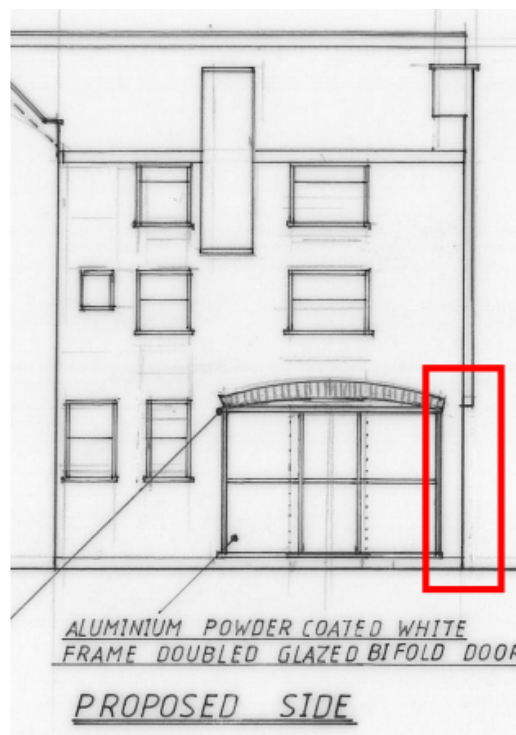
Image 2 – showing side elevation with lower part of chimney breast removed
