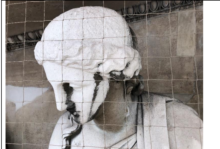
Figure 5: detail showing gypsum crust formed on statue
