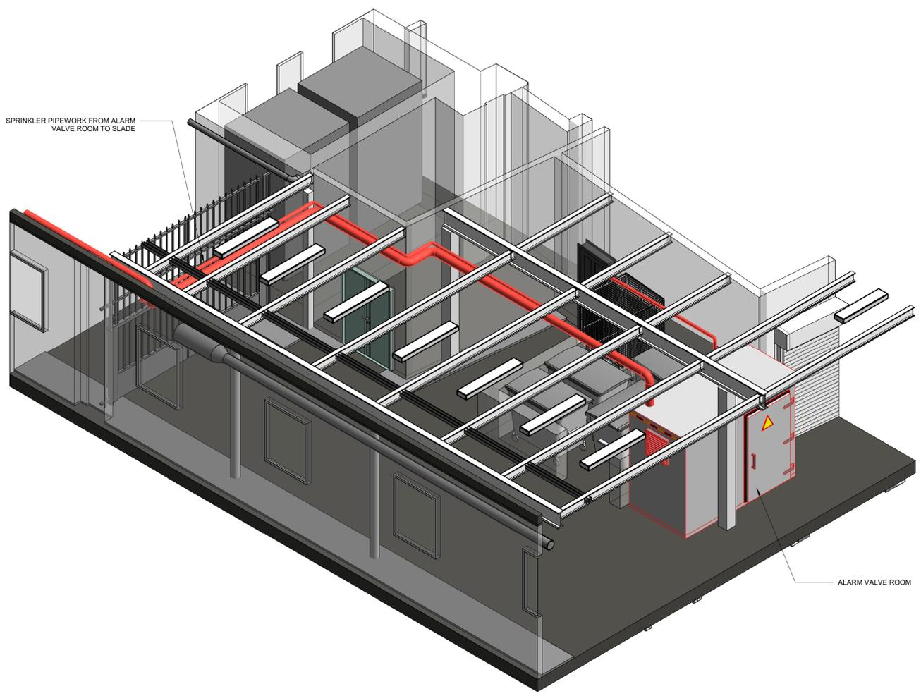
1 Service Yard Alarm Valve Room Sprinkler Pipework Arrangement
