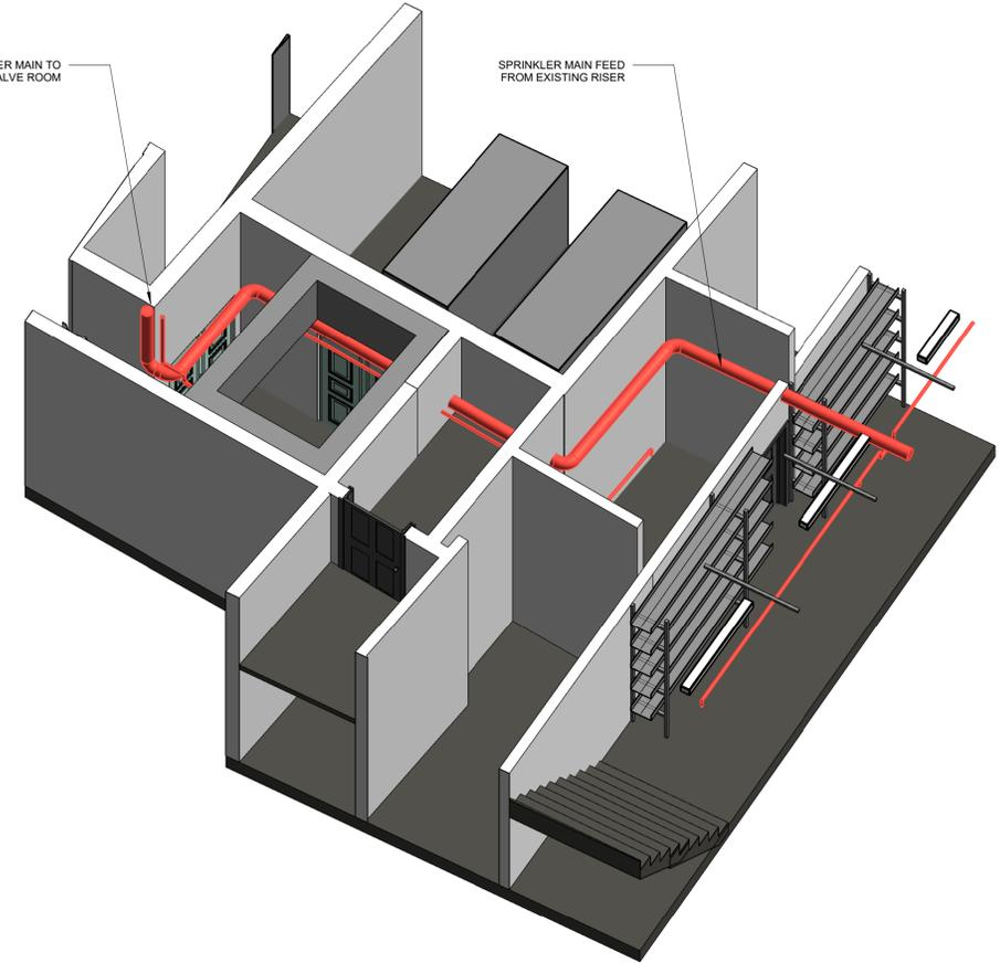
6 Tunnel Pipework to Alarm Valve 3D 2
