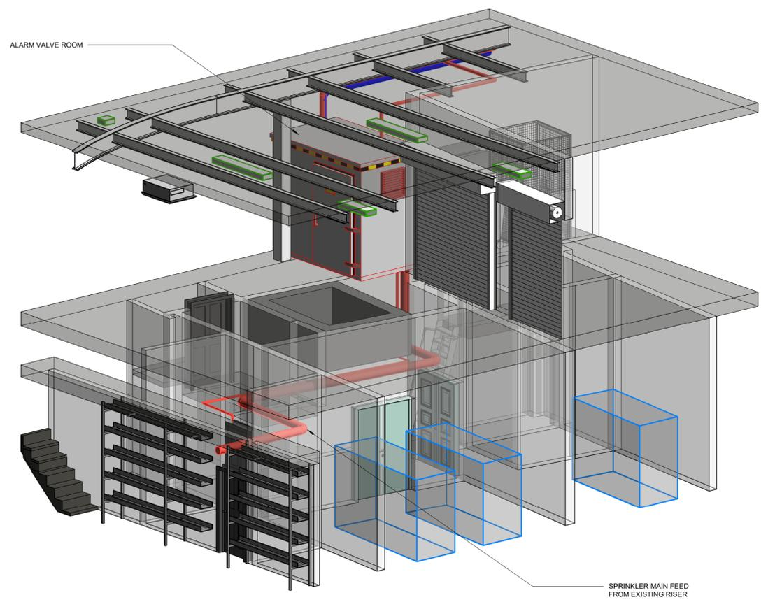
2 Tunnel Pipework to Alarm Valve Room 3D 1
